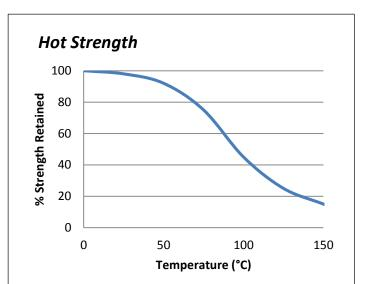
"Hot strength" shear strength tests performed on mild steel. Fully cured then conditioned to pull temperature for 30 minutes before testing. MS359A GREY can withstand higher temperatures for brief periods (such as for paint baking and wave soldering processes) providing the joint is not unduly stressed. The minimum temperature the cured adhesive can be exposed to is -40°C (-40°F) depending on the materials being bonded.
